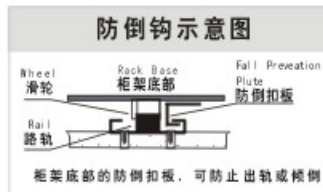
斜坡地面式轨道断面图 Sectional drawing of sloping land track sets
